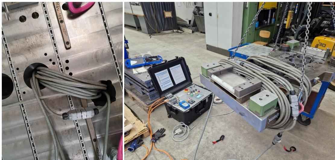
With additional strong pulse coils for demagnetization, tool surfaces can also be demagnetized directly in the presses without having to remove them. Medium and small components can be demagnetized particularly effectively with tunnel coils of the SSM series.
